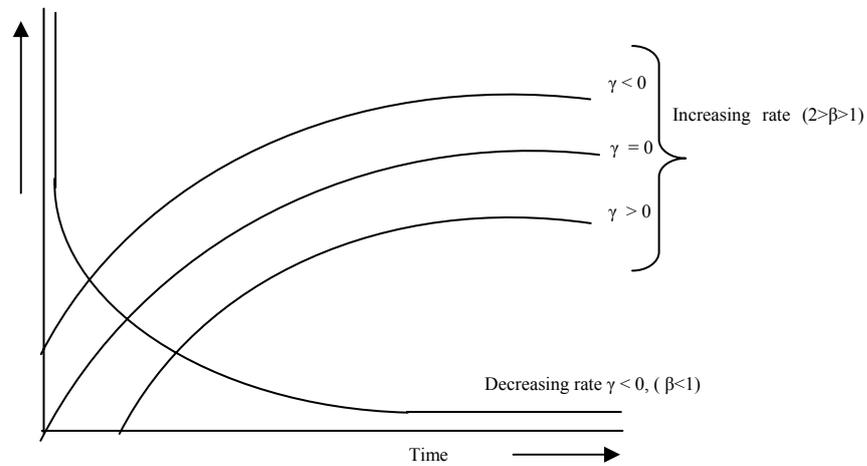
Figure 2.2 Rate of deterioration-time relationship for three-parameter Weibull distribution
