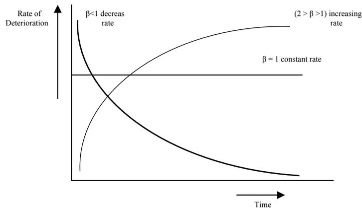
Figure 2.1 Rate of deterioration-time relationship for a two-parameter Weibull distribution
