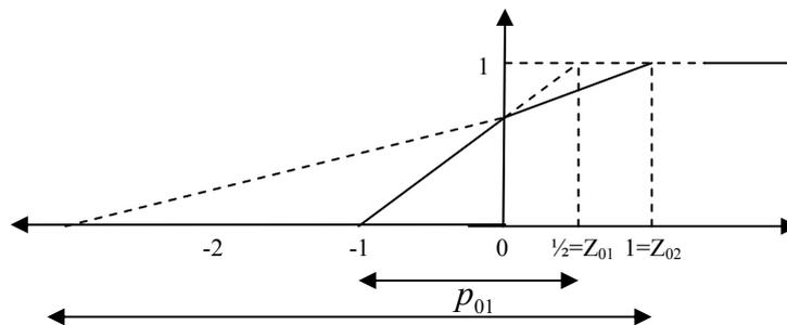
**Figure 2:** Piecewise linear membership functions for problem (P)
