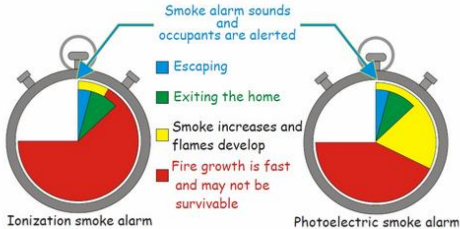
Figure 1: Ionization vs. Photoelectric smoke alarms
