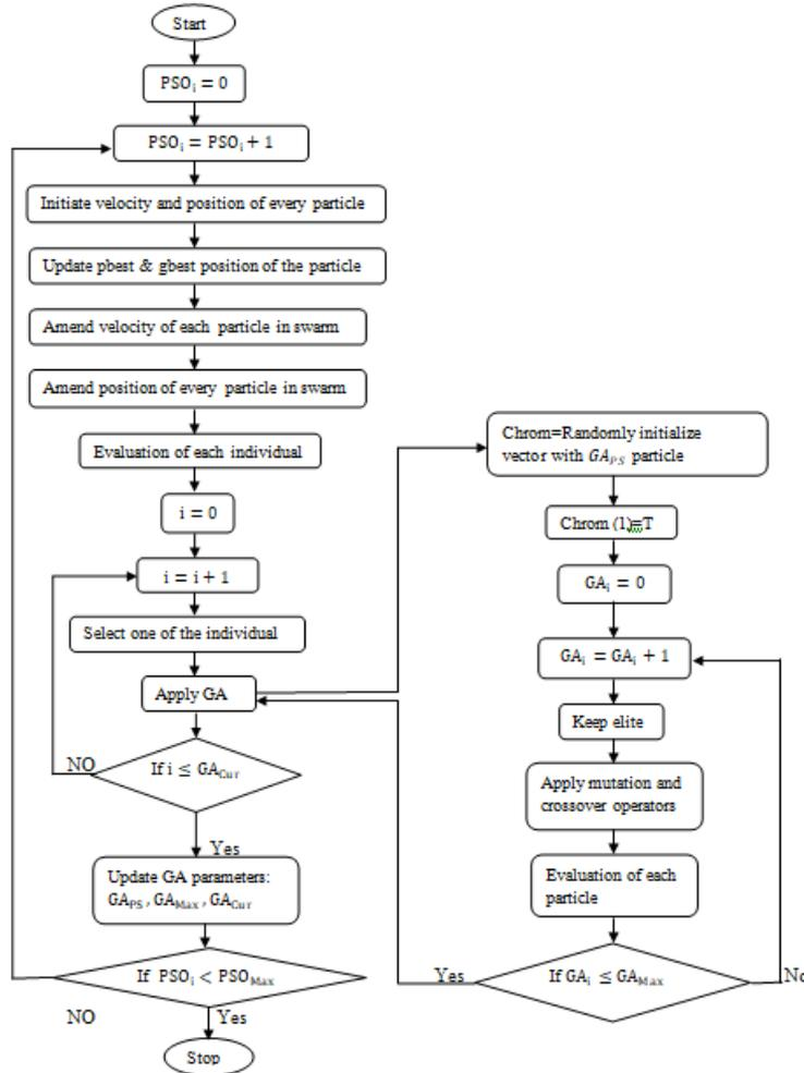
Figure 2: Flow chart for genetic algorithm
