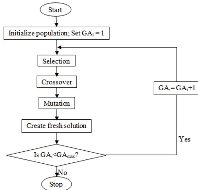
Figure 1: Flow chart for genetic algorithm
