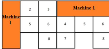
Figure 5: The horizontal or vertical placement of different sized machines in the layout
