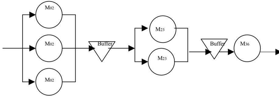
**Figure 1:** Schematic diagram showing a flexible production line.
